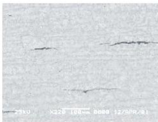
Figure 1. Hydrogen induced cracks (ASTM 515(60) Steel plate) (AIT Advanced Inspection Technologies)
