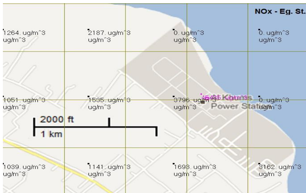
Figure 4. Illustrates the accumulation of nitrogen oxides at Al-Khoms power station under calm atmospheric conditions when emitting quantities equivalent to the maximum limit value of the Egyptian standards.
