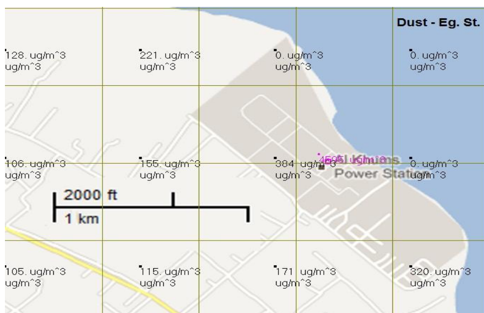
Figure 6. Illustrates the accumulation of solid particles at the Five Power Station when the ambient air is calm and emissions are equal to the maximum allowable limit according to the Egyptian standards
