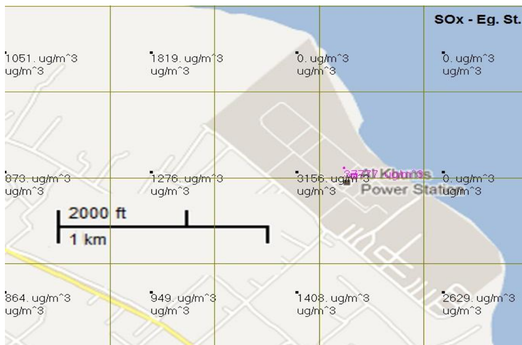
Figure 2. Illustrate the accumulation of sulfur dioxide at Al-Khoms power station under calm atmospheric conditions when emitting quantities of sulfur dioxide that are equivalent to the maximum limit value of the Egyptian standards.
